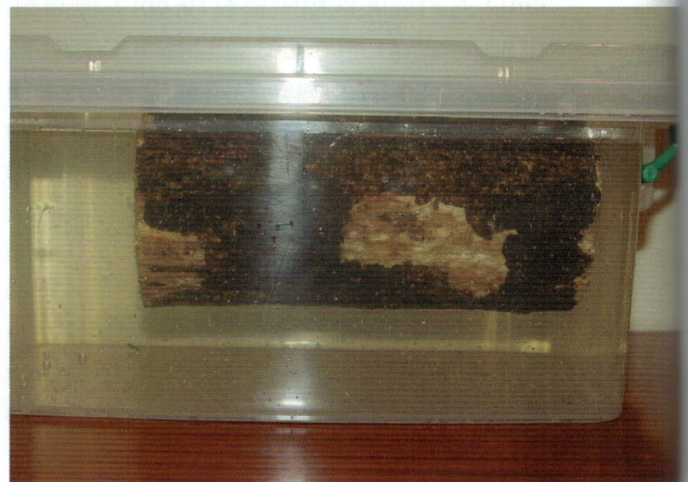
↗加蓋後完全泡水。 Complete submergence with lid.
