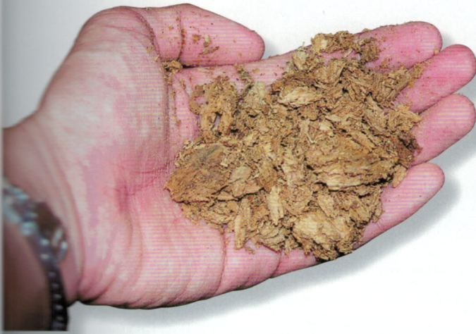
↓ 軟朽木用手隨便一揉便變為軟朽木屑。2000 Soft decayed wood can be converted into flakes with bare hands.
